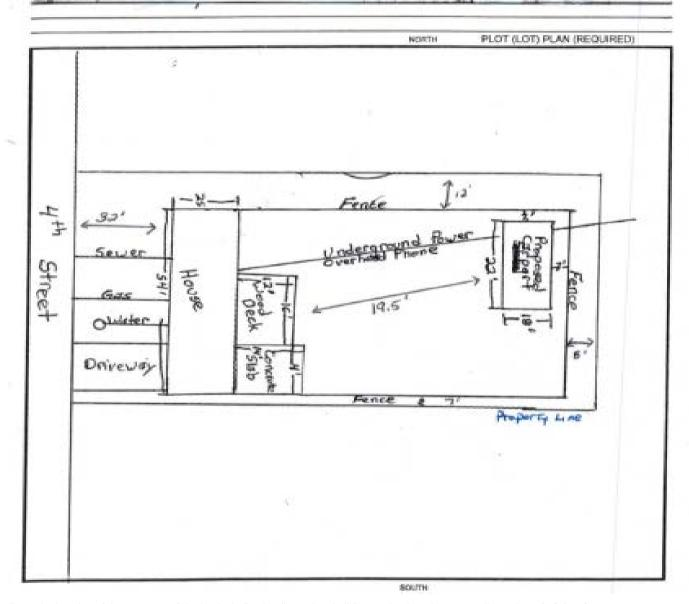
1. Indicate the location of the structure of the lot, including lot dimension, building set back and structrue dimensions, **height of structure**, street name, location of sewer line, gas line, water line and any buried cables. Proberty pins must be located and marked
